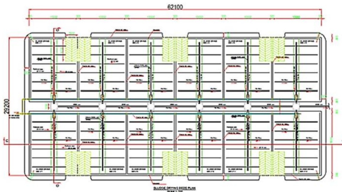
Figure 10: Proposed Sludge drying Bed (phase 1)
