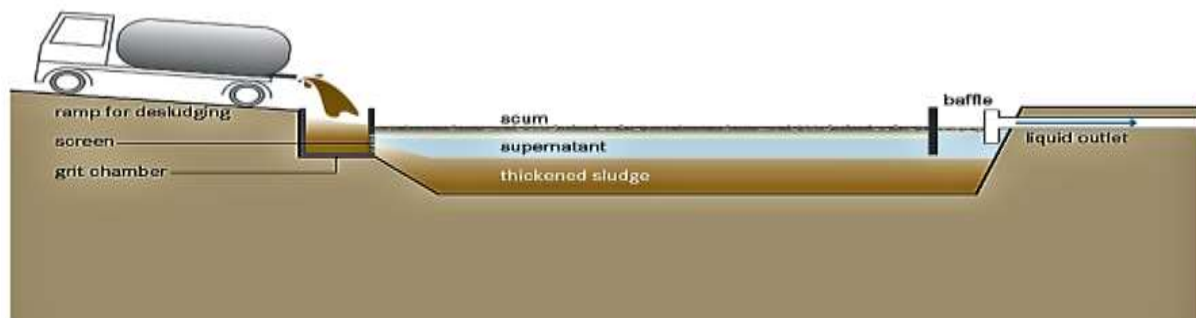
Figure 20 Schematic of a Thickening pond
